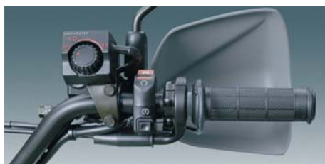
⑩ Grip Heater Kit ⑪ Sub Harness + ⑫ Sub Harness - Flexible, adjustable grip heater to warm fingers on cold winter mornings. The grip heater incorporates a plate that heats the underside of the grip. Integrated circuit to protect the battery from drain. For connection you should purchase items 11 and 12. Item 13 is only required for CB600F.
