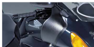
12 Knuckle Visor Set of two, plastic knuckle visors that easily attach to front upper cowi. Further enhances rider protection from bad weather.
