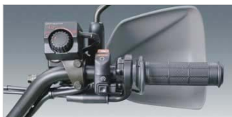
14 Grip Heater Kit 15 Sub Harness + 16 Sub Harness - Flexible, adjustable grip heater to warm fingers on cold winter mornings. The grip heater incorporates a plate that heats the underside of the grip. Integrated circuit to protect the battery from drain. For connection you should purchase items 15, 16, 17 and 18.
