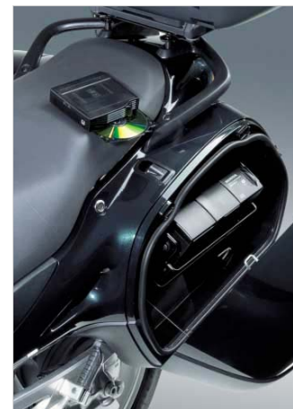
25 CD Changer A Pioneer six CD player with electronic skid protection system and direct disc loading. CD changer neatly fits into the left hand side pannier, where it is protected against dust and water. Not easily accessible to avoid theft.
