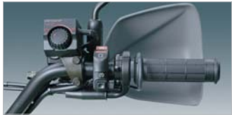
21 Grip Heater Kit 22 Sub Harness + 23 Sub Harness - Flexible, adjustable grip heater to warm fingers on cold winter mornings. The grip heater incorporates a plate that heats the underside of the grip. Integrated circuit to protect the battery from drain. For connection you should purchase items 21, 22 and 23.
