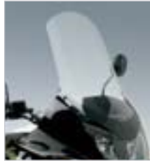
⑬ Tall Windshield 20cm higher, Polycarbonate screen improves wind protection and reduces riding fatigue. An additional stay is concealed underneath the meters avoiding any unpleasant vibrations.
