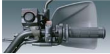
⑭ Grip Heater Kit ⑮ Sub Harness + ⑯ Sub Harness - ⑰ Heated Grip Switch Bracket ⑱ Handle Weight Spacer and Installation Manual Flexible, adjustable grip heater to warm fingers on cold winter mornings. The grip heater incorporates a plate that heats the underside of the grip. Integrated circuit to protect the battery from drain. For connection you should purchase items 15, 16, 17 and 18.
