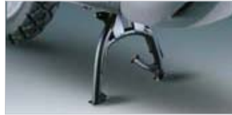
19 Main Stand Conventional centre stand, providing optimal stability on variable ground surfaces, while facilitating rear wheel maintenance.
