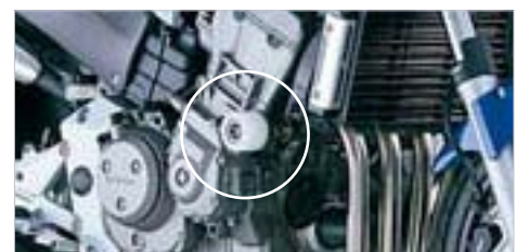
④ Mushroom Engine Guard A set of compact, mushroom-type engine guards like those seen on many of Honda's racing machines, that attach to the engine mounts and feature durable canister-shaped nylon bodies on aluminium shafts with shock-absorbing rubber liners, to protect the engine cases and fuel tank in the event of a fall.
