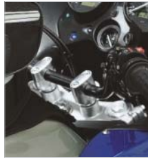
12 Handlebar Bridge Easy to fit aluminium bolt-on bridge, installed to carry a handlebar pocket bag.
