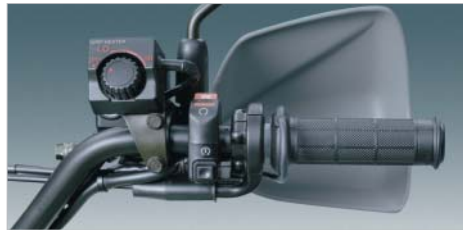
17 Grip Heater Kit 18 Sub Harness + 19 Sub Harness - Flexible, adjustable grip heater to warm fingers on cold winter mornings. The grip heater incorporates a plate that heats the underside of the grip. Integrated circuit to protect the battery from drain. For connection you should purchase items 18, 19 and 20.
