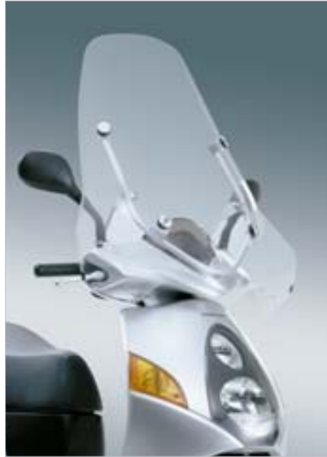
⑬ Windshield 500 x 506 x 4mm Polycarbonate Lexan windshield offering perfect protection against the elements, with integrated hand protectors. Specially designed to ensure utmost vehicle stability, limiting vibration. The rubber, mounted stay allows the shield to fall forward on impact and is WVTA (Whole Vehicle Type Approval) cleared.
