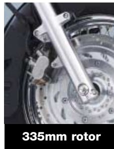
The front disc brake features a twin-piston calliper with large diameter 335mm rotor for excellent stopping power.
