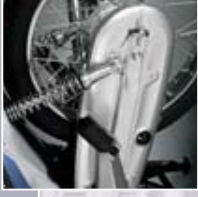
Sturdy pressed-steel chain guard protects vital hardware from the elements and reduces maintenance.
