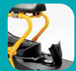
A locking fuel filler cap, built into the rear floor panel, allows refuelling without having to leave the seat.
